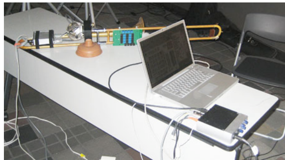
Figure 14: Complete setup for trombone rev. 3, showing loaded trombone, mute, Powerbook, multi-channel audio interface. Tokyo, 2008.
