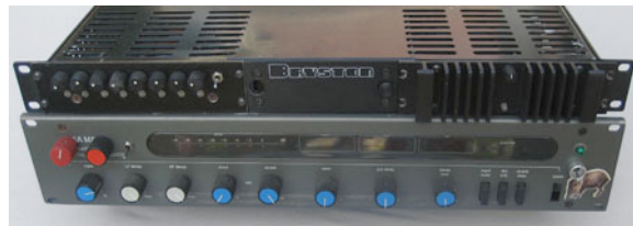
Figure 1: Trombone-propelled electronics rev. 1: modified Stargate below; Bryston 2B-LP chassis above, containing amplifier channel for trombone speaker in right side, computer-controlled 8-input mixer on left (for selecting sound source to process.)
